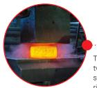
The honeycomb seal begins life as two separate components - pre-annealed steel forgings to create the steel outer ring, and strips of nickel-based superalloy for the honeycomb.
