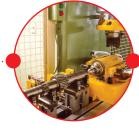
The parts undergo automatic shaft straightening to correct any distortion caused by high processing temperatures.
