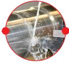
The piston is machined to its final tolerance.
