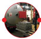
The part is vacuum hardened. This gives the part the strength it needs to withstand demanding in-service requirements.
