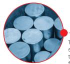
The device begins its journey as steel billet. Quality and purity of the steel is critical - it must be free from inclusions to generate a defect free surface.
