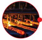
The extruder screw begins life as a forged steel bar.
