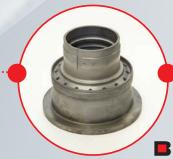
Post-nitriding, the plating and the white layer (nitrogen-rich layer which does not diffuse on to the surface) are removed. Rough machining is carried out, usually to within 1/16th inch of the final part size.
