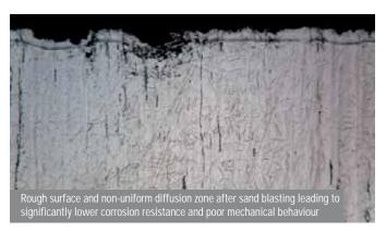
Fig. 3: Comparison of LTSH results for AISI 316L after electropolishing (left) and sand blasting (right). Sand blasting leads to local high deformations with excessive formation of deformation martensite. Diffusion is hindered and corrosion resistance is lowered. In comparision, the electropolished surfaces lead to a defect-free and homogeneous diffusion zone.
