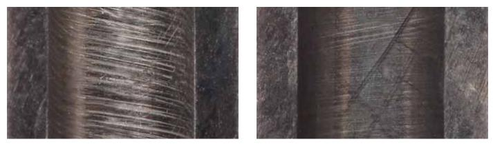
Fig. 4: Honed stainless steel surface. Right: High cutting forces and a worn tool lead to a surface which is rather deformed than cut. Left: low forces and sharp tool lead to distinct grinding patern, which is natural for correct honing operations. Less deformation, heat input and smearing lead to better diffusion behaviour and improved corrosion resistance.
