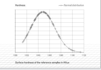
Surface hardness of the reference samples for the S<sup>3</sup>P K22 process during one calendar year; Results for one Kolsterising<sup>®</sup> unit; the minimum surface hardness of 1000 HV0.05 was reached safely in all treatments.
