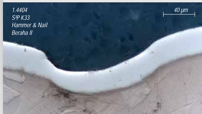
Fig. 2 316 (1.4404) stainless steel sample, impact of hammer and nail test showing good deformability.
