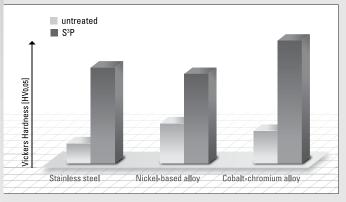
Comparing the surface hardness, S<sup>3</sup>P treated materials show higher levels of hardness, resulting in improved wear resistance.
