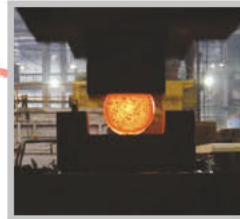
Alloy steel billet is forged to shape.
