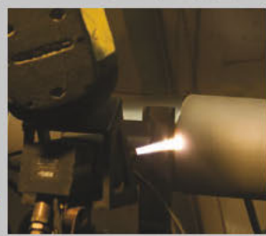
B A thermally sprayed surface treatment is applied to replace hard chrome plate for improved wear and corrosion resistance.
