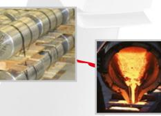
The billets are investment cast to form the blade shape and then fettled to remove casting material.
