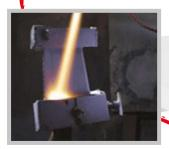
A thermally sprayed coating is applied to improve temperature resistance.
