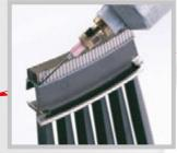
Honeycomb for abradable seals is vacuum brazed onto the vanes' main sections.
