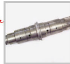
The forged steel part is then machined into its near net shaft shape and sent for heat treatment.
