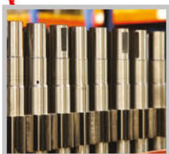
The shafts are machined again to achieve final engineering dimensions.
