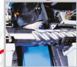
The steel is then machined into the rotor shape required for down-hole drilling.
