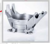
The component is then removed from its build plate by electrical discharge machining (EDM) to prepare for HIP and heat treatment.
