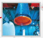
Hot Isostatic Pressing (HIP) ensures that any porosity within the part is removed, thereby reducing the variation in mechanical properties when compared with the as-built part, and improving ductility and fatigue strength.
