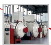
The part is stress relieved in a vacuum furnace to minimise any distortion.
