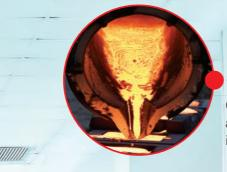
Cobalt chromium alloy billets are precision cast to form implant shape.
