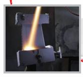
A thermally sprayed coating is applied to improve temperature resistance.
