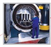
Honeycomb for abradable seals is vacuum brazed onto the vanes' main sections.
