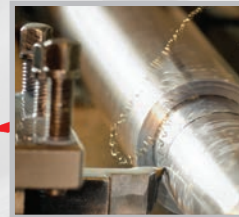
Rough machining is carried out, usually to within 1/16th inch of the final part size.
