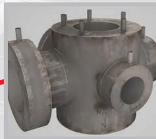
The fabricated capsule, almost identical in shape to the finished component but larger in size, is filled with powder.
