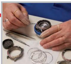
The individual watch components – up to 300 parts – are manually assembled.\*
