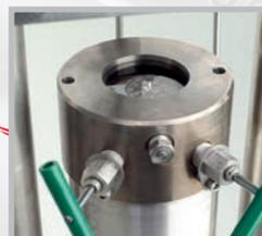
The watch is tested for performance – a diving watch, for example, must withstand a 125 bar (nominal) pressure test.\*
