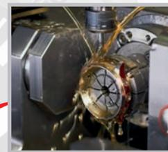
The case – a complex 3D shape – is machined from a disc or circular blank to tight tolerances, to meet the demands of specification and functionality.\*
