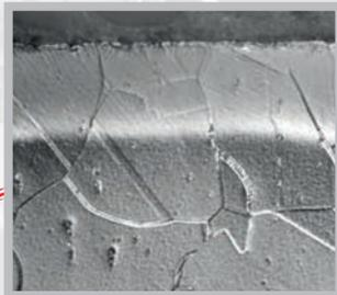
Bodycote's S<sup>3</sup>P technology is applied to bezels, cases and straps to provide an exceptionally wear and scratch resistant surface. The hardening process has no negative effect on the appearance or natural corrosion resistance of the steel.
