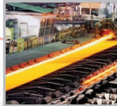
The rotors begin life as pieces of steel bar.
