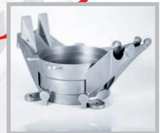
The component is then removed from its build plate by electrical discharge machining (EDM) to prepare for HIP and heat treatment.
