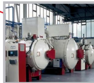
The part is stress relieved in a vacuum furnace to minimise any distortion.
