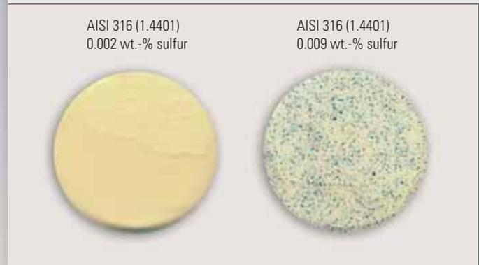
*Fig. 1 Material, AISI 316 (1.4401); Passive layer tested by KorroPad (BAM); left: sulfur content 0.002 wt %; stable and uniform passive layer; right: sulfur content 0.009 wt %; finely distributed manganese sulfides form weak points in the passive layer; by J. Lehmann, A. Burkert; Federal Institute for Materials Research and testing; 17136 N / 1 GfKORR; 2014.*
