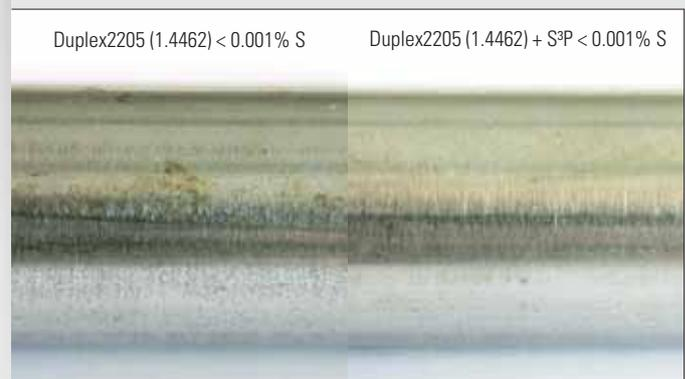
*Fig. 2 Material 1.4462; after 672 h salt spray test; left: solution-annealed at 1050 °C / 1 h; right: solution-annealed at 1050 °C / 1 h + S<sup>3</sup>P-treated; investigation conducted by UGITECH-CRU.*
