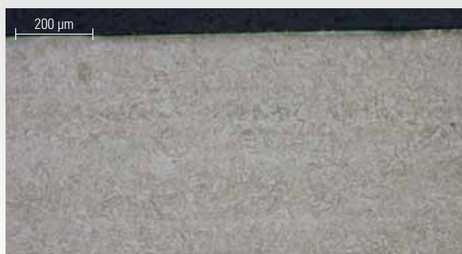
Microstructure of a S 3 P-treated 15-5PH (1.4545) after 720 hours in a sour gas atmosphere at 120 °C under mechanical stress. No signs of stress corrosion.
