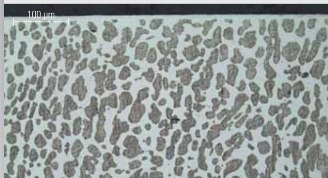
Microstructure of a S 3 P-treated 1.4462 (AISI 316L) after 720 hours in a sour gas atmosphere at 90 °C under mechanical stress. No signs of stress corrosion.
