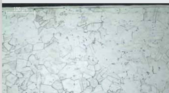
Microstructure of a S 3 P-treated 1.4404 (AISI 316L) after 720 hours in a sour gas atmosphere at 149 °C under mechanical stress. No signs of stress corrosion.
