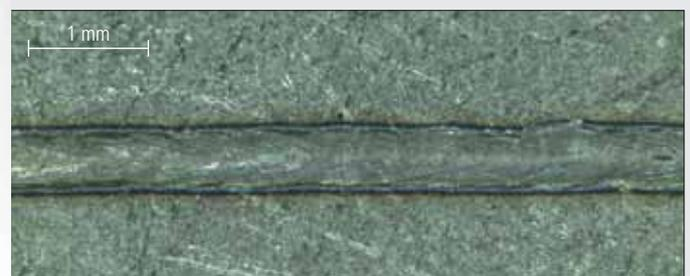
Fig. 3 Weld track of low temperature carburized stainless steel after pickling and passivation; the corrosion resistance was measured to be on the same level as the base material.
