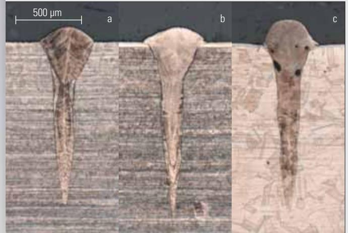
Fig. 1 Cross section of single mode fiber laser weldments on AISI 316L stainless steel ( $P: 500\text{ W}$ ;  $v: 100\text{ mms}^{-1}$ );
