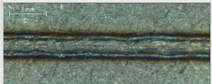
Fig. 2 As welded surface of low temperature carburized stainless steel; massively lowered corrosion resistance mainly due to heat tint.
