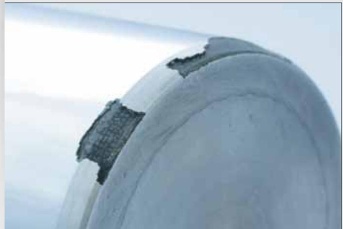
Fig. 2 Hard chrome-plated cylinder with flaking due to dynamic stress; this problem does not exist with S<sup>3</sup>P treated surfaces.
