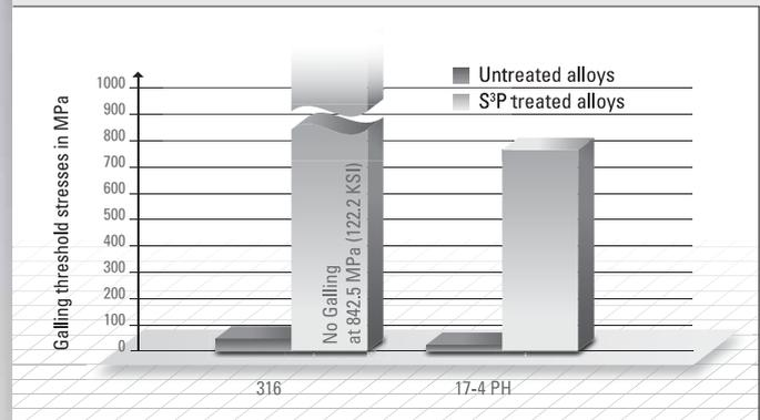
Fig. 1 Galling resistance of materials, ASTM G98 testing; threshold galling stress of untreated and S<sup>3</sup>P treated materials.
