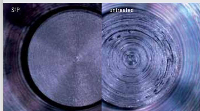
Fig. 2 Photographs of AISI 316 buttons after G98 galling test. Left: S<sup>3</sup>P treated condition at 842.5 MPa (122.2 KSI), no galling; right: untreated condition at 45.5 MPa (6.6 KSI), galling.
