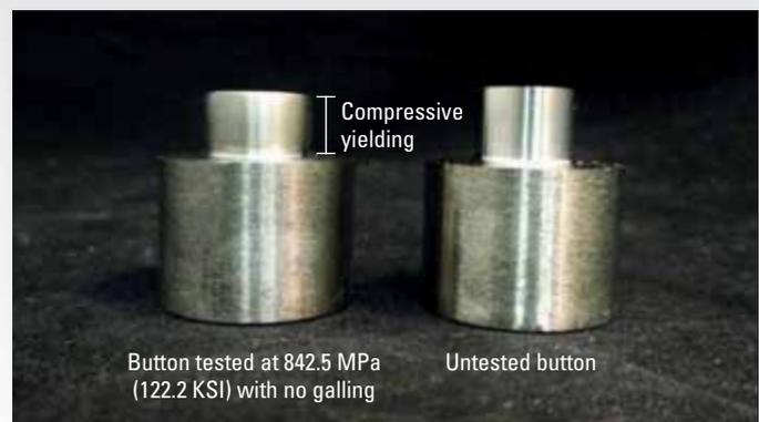
Fig. 3 Photo of AISI 316 button tested at 842.5 MPa (122.2 KSI) resulting in compressive yielding; no galling was observed.
