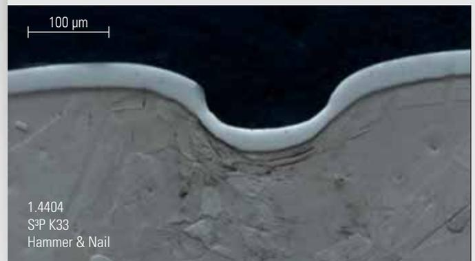
Fig. 2 No cracks visible in heavily deformed carbon S-Phase after hammer & nail test of S<sup>3</sup>P treated AISI 316L.
