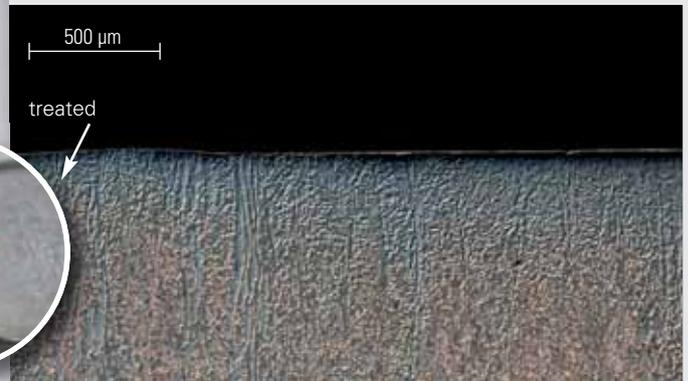
S<sup>3</sup>P-treated Duplex2205 (1.4462) after cavitation testing in accordance with ASTM G32-10 (27h).
