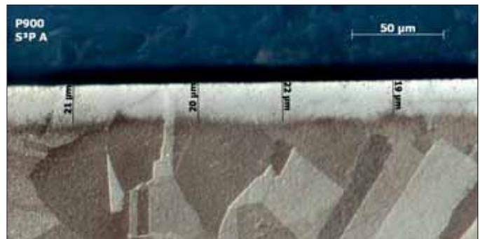
Microstructure of special steel P900 (1.3815), S<sup>3</sup>P A treated with a diffusion depth of 19 - 22 µm
