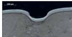
Cross section of treated stainless steel AISI 316L after rapid heavy deformation (hammer & nail test)
