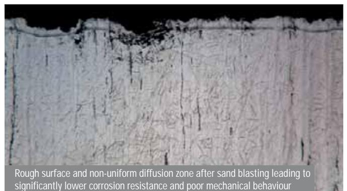
Rough surface and non-uniform diffusion zone after sand blasting leading to significantly lower corrosion resistance and poor mechanical behaviour
