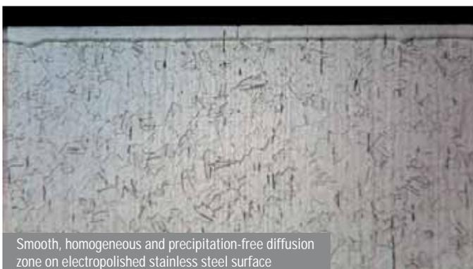
Smooth, homogeneous and precipitation-free diffusion zone on electropolished stainless steel surface
