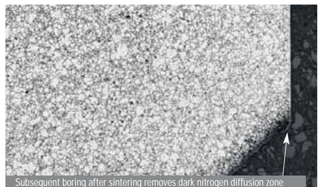
Fig. 6: Cross section sintered, stainless steel MIM parts. Nitrogen diffusion (dark surface area) prevents unhindered diffusion and high surface hardness after LTSH. A subsequent boring operation (right) removes the nitrogen diffusion zone partially. Unhindered diffusion is possible in this region.
