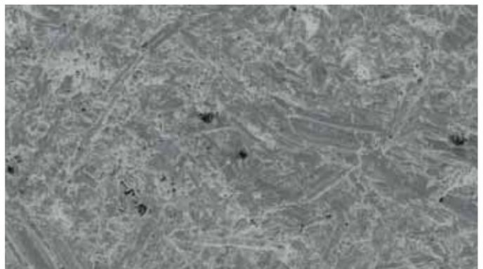
Fig. 2: Stainless steel surface after vibratory finishing. Left: smooth surface (Ra 0.17) with little defects, achieved with adjusted parameters and soft abrasives. Right: coarse surface finish (Ra 0.56), abrasive inclusion and excessive formation of deformation martensite, which leads to poor corrosion and diffusion behaviour.
