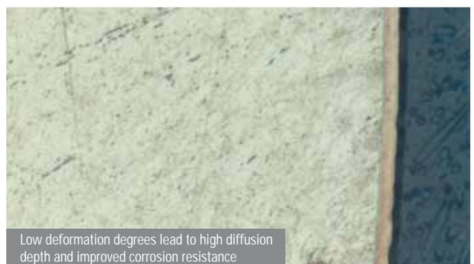
Fig. 5: Surface hardened stainless steel component. Left: Punched surface. Irregular and heavily deformed (dark areas) surface. Lowered diffusion depth and impaired corrosion properties in this zone. Right: same part bored instead of punched. Less deformation and regular surface finish lead to higher diffusion depth and improved corrosion properties.
