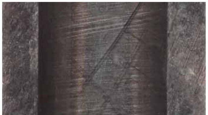
Fig. 4: Honed stainless steel surface. Right: High cutting forces and a worn tool lead to a surface which is rather deformed than cut. Left: low forces and sharp tool lead to distinct grinding pattern, which is natural for correct honing operations. Less deformation, heat input and smearing lead to better diffusion behaviour and improved corrosion resistance.
