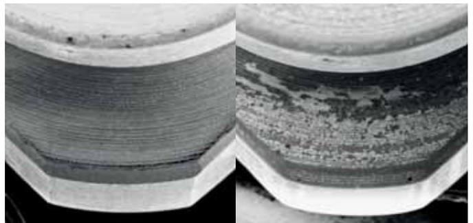
*Fig. 1: Turned stainless steel surface. Left: sharp tool and adjusted machining parameters lead to a regular surface finish. Right: worn tool and high cutting forces lead to smearing of the surface/ irregular finish with reduced corrosion resistance, flaking and poor diffusion behaviour.*
