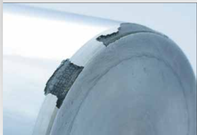
Fig. 2 Hard chrome-plated cylinder with flaking off due to dynamic stress; this problem does not exist with S 3 P-treated surfaces.
