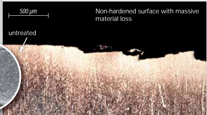
Untreated Duplex2205 (1.4462) after cavitation testing in accordance with ASTM G32-10 (27h).
