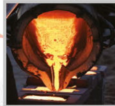
Cobalt chromium alloy billets are investment cast to form implant shape.
