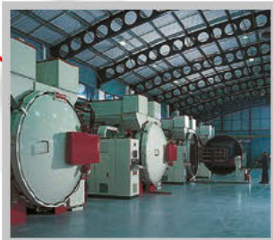
Solution and ageing heat treatment is used to strengthen the implant.
