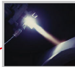
The castings are thermally sprayed with a biomedical coating to allow a bond to form between the implant and body tissue, promoting bone growth.
