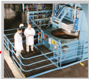
The implants are then HIPed to eliminate porosity, improve fatigue life and enhance the bonding of the biocompatible coating.
