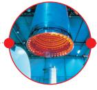
The implants then undergo Hot Isostatic Pressing to eliminate porosity, improve fatigue life and enhance the bonding of the biocompatible coating.
