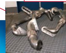
Fluid tube, vacuum brazed, and heat treated
