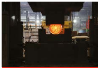
Alloy steel billet is forged to shape.
