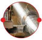
Rough machining is carried out, usually to within 1/16th inch of the final part size.
