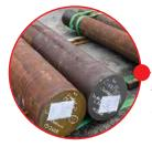
The cylinders start life as solid high strength steel rods.
