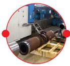
The solid steel rods are machined into hollow cylinders.
