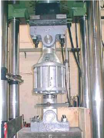
High load test on bridge damper
