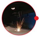
The metal part is 'built' onto a plate in a 3D printing machine by depositing metal powder in layers which are then consolidated, for example using lasers.
