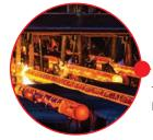
The extruder screw begins life as a forged steel bar.
