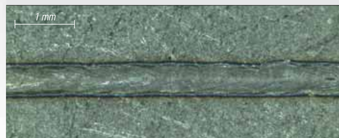
Fig. 3 Weld track of low temperature carburised stainless steel after pickling and passivation; the corrosion resistance was measured to be on the same level as the base material.
